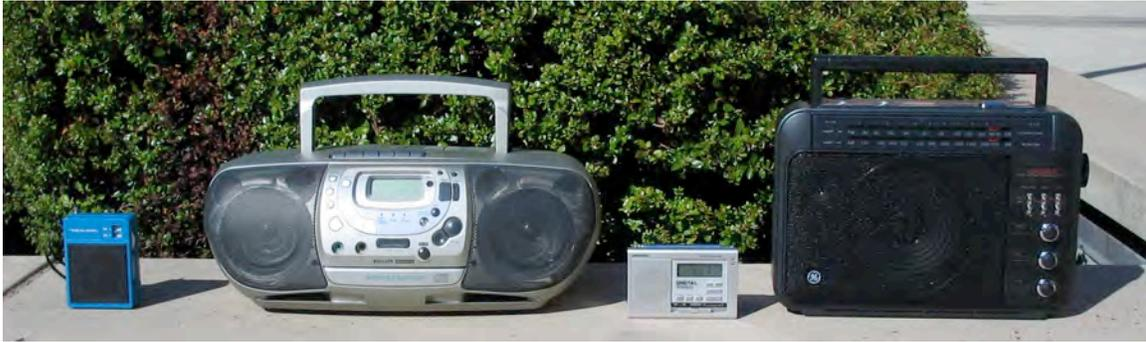
**Fig 2: A Succession of Radios.** Several radios were tried in an attempt to get a strong AM audio signal. The GE SuperRadio on the right is specially designed to receive weak signals.
