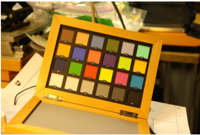
This is the input image with wrong colors because of fluorescent lamp.
