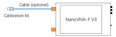
Tap on **[OPEN]**, the device emits a beep, and the menu turns gray and is inoperable. Wait for 2-3 seconds, the device emits a beep again, an  $\square$  marker will appear ahead of "OPEN", and a letter "O" appears at the bottom of the screen, indicating that open calibration is finished.
