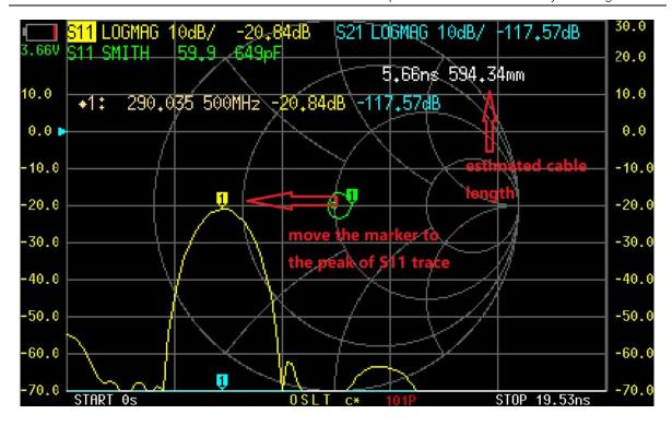
There are 3 kinds of digital processing mode available: **[LOW PASS IMPULSE]**, **[LOW PASS STEP]**, **[BANDPASS]**, and default setting is **[BANDPASS]**.
