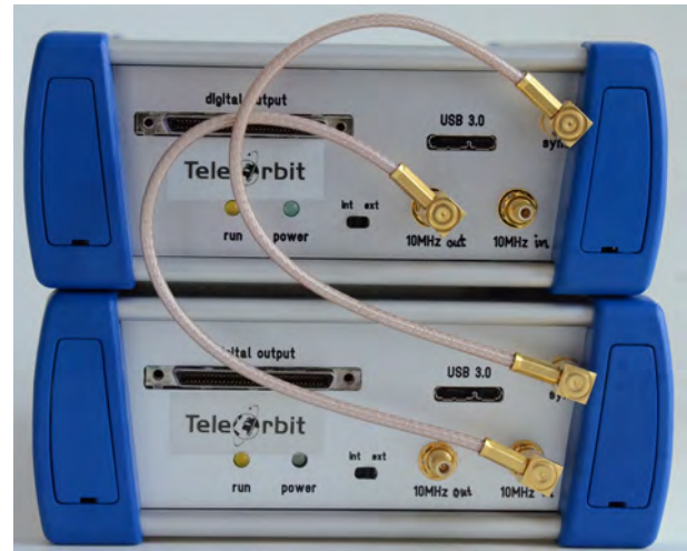
Figure 9. Synchronization of two Flexiband USB 3.0 units
