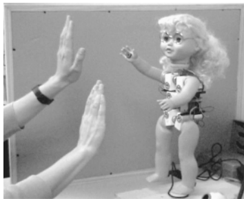
Figure 1. Robota, a minihumanoid, doll-like robot, can mirror the arm and head motion of a human demonstrator by visual tracking of the optical flow. Researchers are investigating its use as an educational toy for normal and handicapped children. (From Billard in Dautenhahn, K., and Nehaniv, C., Eds., 2002, Imitation in Animals and Artifacts , Cambridge, MA: MIT Press, Reproduced with permission.)
