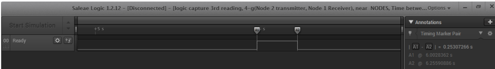
Figure 6.17: Time between consecutive toggles on the READY event at sampling rate 100 MS/s for 10 seconds duration
