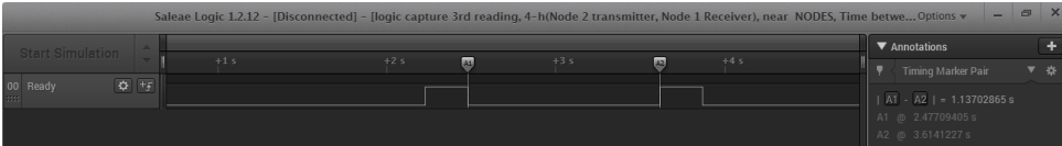
Figure 6.18: Time between consecutive toggles on the READY event at sampling rate 100 MS/s for 5 seconds duration
