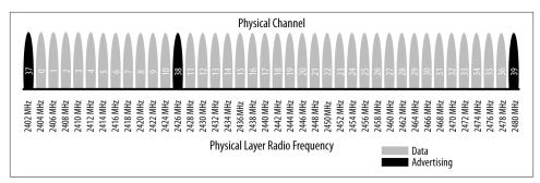
Figure 2-2. Frequency channels
