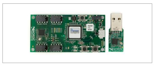
Figure 5-1. Nordic Semiconductor's nRF51822-EK
