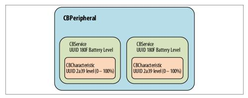
Figure 9-2. Relationship of CBPeripheral, CBServices, and CBCharacteristic objects
