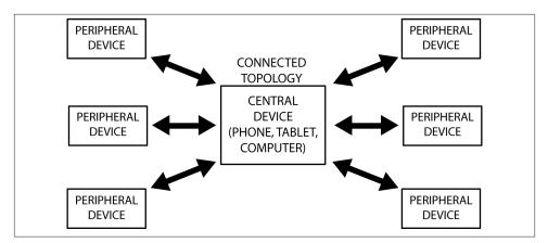
Figure 1-4. Connected topology
