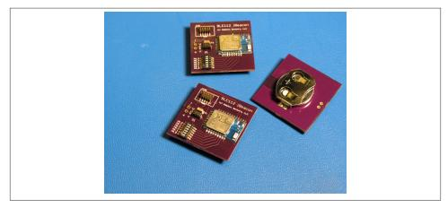
*Figure 9-4. BLE112 modules programmed as iBeacons and powered by CR2032 coin cells.*
