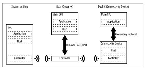
Figure 1-2. Hardware configurations
