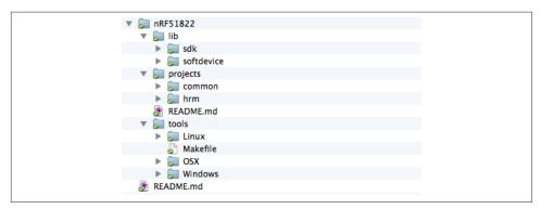
Figure 10-3. Bare file structure for the nRF51822 codebase
