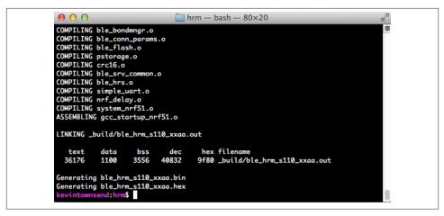
Figure 10-5. Successful cross-compilation and linking using GCC
