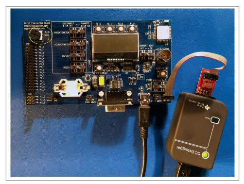
Figure 9-1. Bluegiga BLE112 development breadboard
