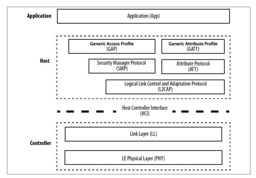
Figure 2-1. The BLE protocol stack
