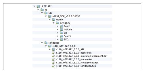
Figure 10-4. File structure for Nordic's SDK and SoftDevice
