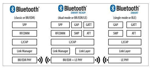
Figure 1-1. Configurations between Bluetooth versions and device types
