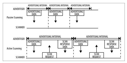
Figure 2-4. Active and passive scanning
