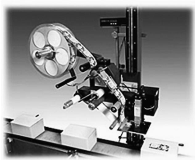
Figure 9.4 An Example of a Wipe-On Label Applicator ( Image Courtesy of Weber Marking Systems Inc. )
