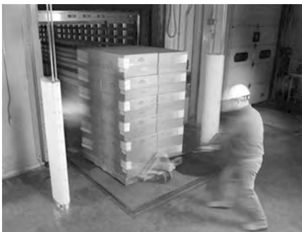
Fig. 7.3. Typical RFID enabled warehouse loading bay portal.
