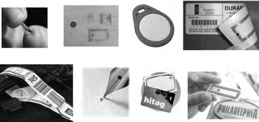
Fig. 1.2. A collection of RFID tags using inductive coupling in different form factors and packagings.
