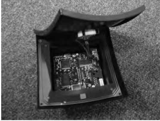
Fig. 4.2. A conductor loop antenna used by the Philips Pagoda reader, which employs the magnetic component of the radio wave for energy transfer and communication with tags.
