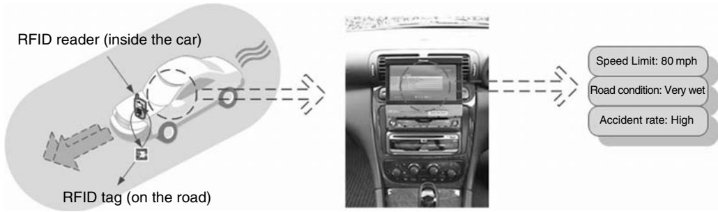
FIGURE 22.11 Advanced road information system architecture.
