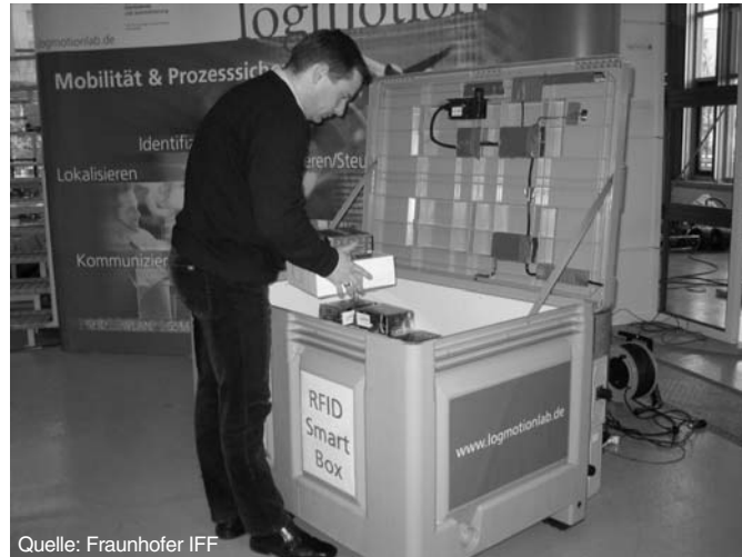
Figure 7.16 A container with an e-seal, RFID antenna and GPS positioning system (source: Fraunhofer IFF)
