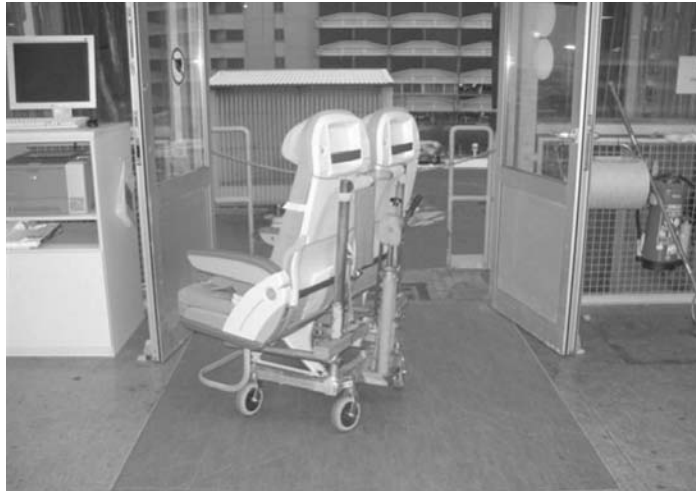
Figure 10.11 Quick-Change seating unit on a floor antenna in front of a loading door [Walther06]
