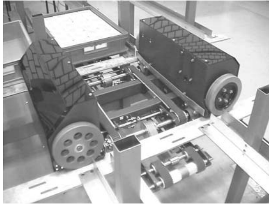
Figure 10.18 Warehouse rail vehicle in an aisle with small-load carriers (source: Fraunhofer IML)
