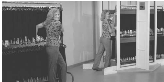
Figure 10.16 Garment rack shipping unit being read while passing through an antenna gate (source: gardeur)
