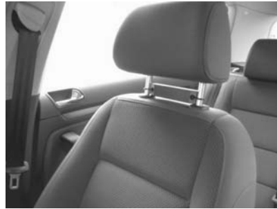
Figure 10.4 A RFID transponder fitted between headrest supports (source: Dat Autohus)
