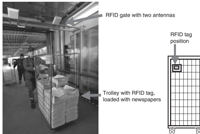
Figure 10.13 A wire-mesh trolley with RFID tags passing through an RFID antenna gate of the Finnish Post Office (source: BEA)
