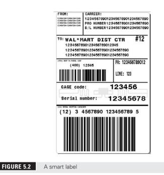
The label should be large enough to display all of the existing printed information as well as any additional information required for the RFID tag embedded in the back of the label, such as the Electronic Product Code (EPC) logo to indicate the use of an EPC tag within the label.
