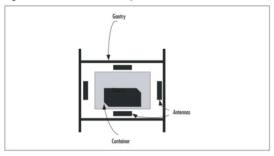
Figure 6.4 The Front View of a Conveyor Portal
