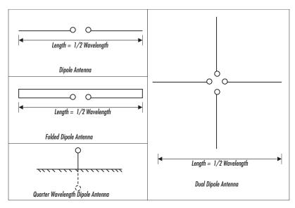
Figure 6.2 Various Kinds of Dipole Antenna
