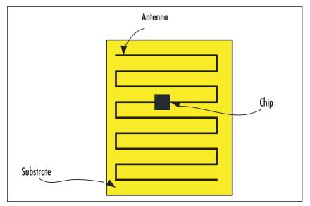
Substrate This is the layer that houses the chip and the antenna. In other words, it's the support structure for the tag. Substrates can be made of different materials such as plastic, polyethylene terephthalate (PET), paper, and glass epoxy. Substrate material can be rigid or flexible, depending on the usage requirements.
