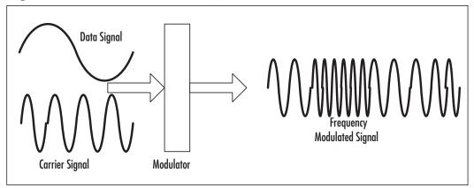
Figure 2.5 An Example of Frequency Modulation
