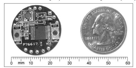
Figure 1.5 A Reader and a Tag: Skyetek's M1-mini (Image courtesy of Skyetek)
