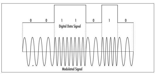
Figure 2.6 An Example of Frequency Shift Keying
