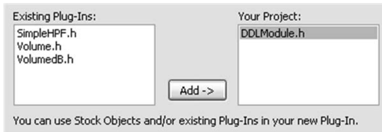
Figure 7.30: Adding existing modules can be done programmatically through RackAFX.
