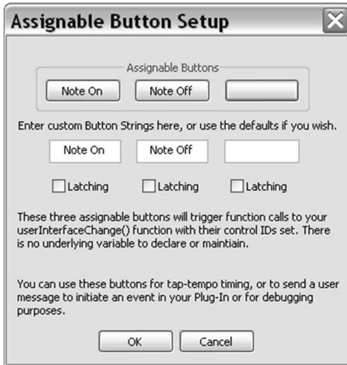
Figure 9.6: The assignable button setup; notice that the last button is blank. RackAFX will hide it when you load the plug-in.
