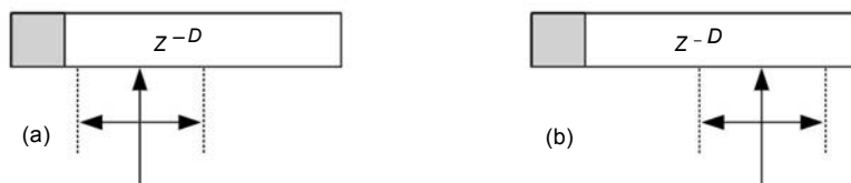
Figure 10.8: (a) and (b) are two different chorus modules with the same maximum depth (dotted lines) but a different center of operation.
