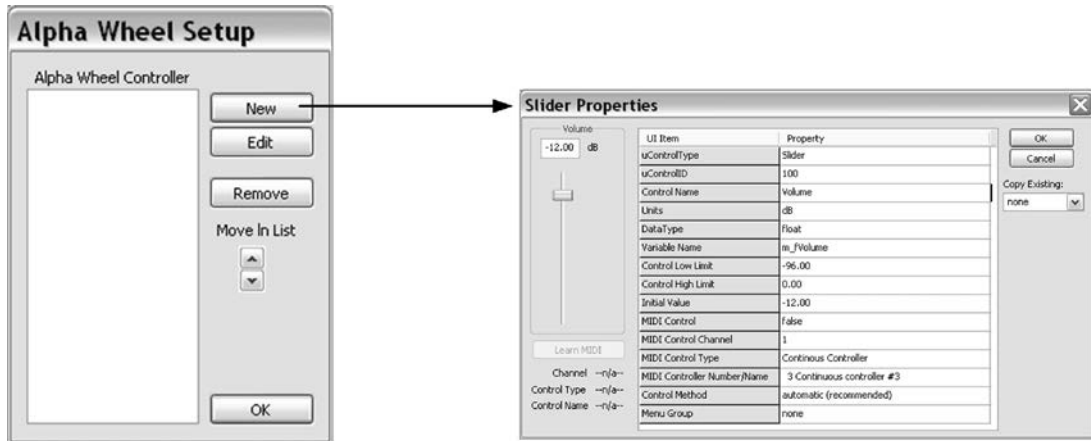
Figure B.1: The New button pops up the slider properties to add a control to the LCD.
