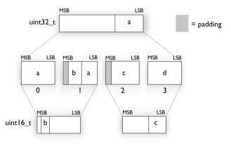
In big-endian mode, each bitfield is allocated starting from the most significant free bit of its container to ensure that it is placed into bytes from left to right.
