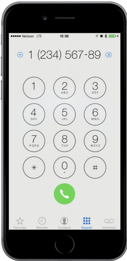
Figure 6-2. The Phone application provides an example of a multiview application using a tab bar
