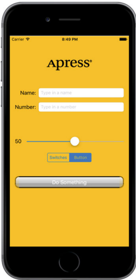
Figure 4-2. Tapping the segmented controller on the left side causes a pair of switches to be displayed. Tapping the right side causes a button to be displayed, as shown here
