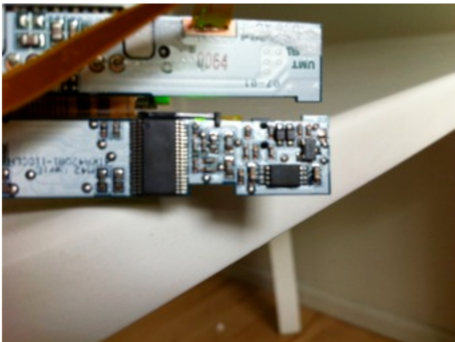
Figure 7: The larger chip is the bq20z80. The next biggest is the bq29412.
