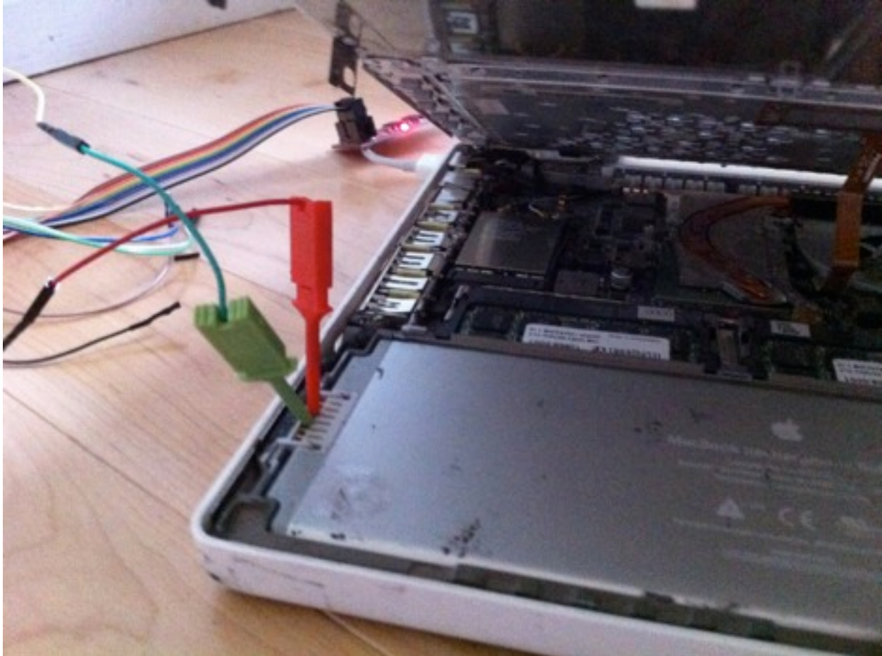
Figure 10: Sniffing the battery to host communications
