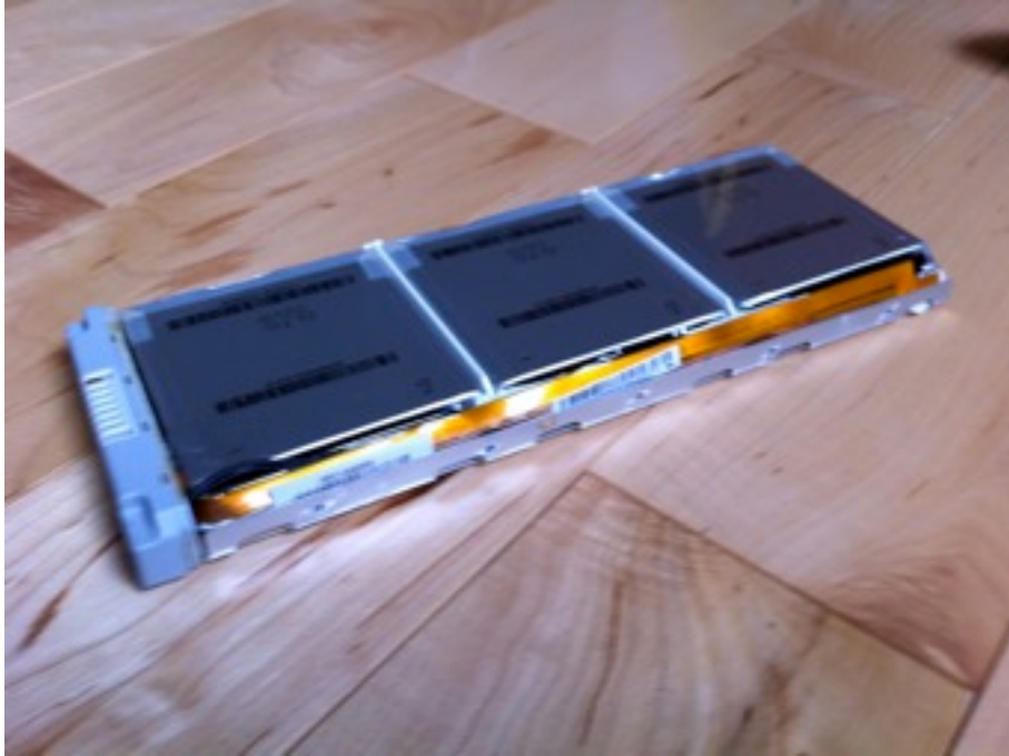
Figure 4: 6 Lithium Polymer cells inside. The electronics are on the end.
