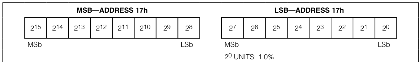
Figure 19. Cycles Register Format (Output)
