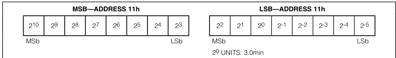
Figure 17. TTE Register Format (Output)
