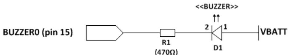
Figure 35. Example of LED Driven by the Buzzer Output
