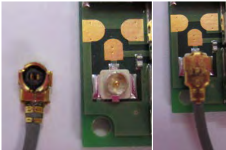
Figure 27. UFL Connector for use with a GSM/WCDMA Antenna
