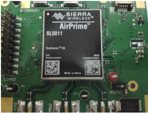
Figure 70. AirPrime SL501x Socket Board Configuration for Current Consumption Measurement
