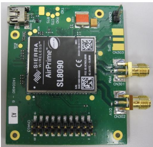
Figure 5. AirPrime SL80xx Socket Board with the AirPrime SL8090 Embedded Module (Top View)
