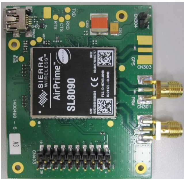
Figure 69. AirPrime SL80xx Socket Board Configuration for Current Consumption Measurement
