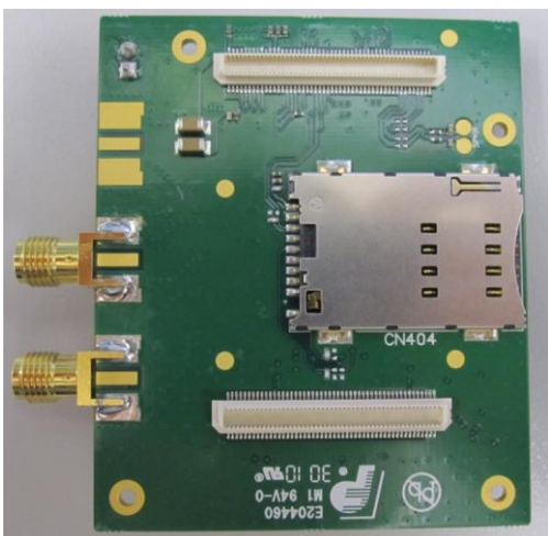
Figure 6. AirPrime SL80xx Socket Board with the AirPrime SL8090 Embedded Module (Bottom View)
