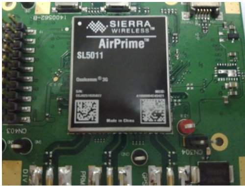
Figure 7. AirPrime SL501x Socket Board with the AirPrime SL5011 Embedded Module (Top View)
