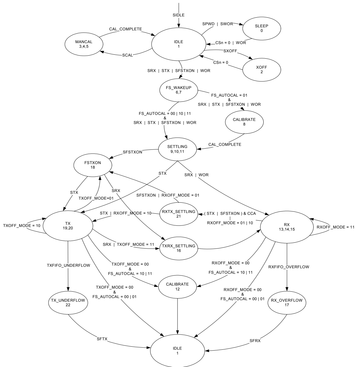
Figure 21: Complete Radio Control State Diagram
