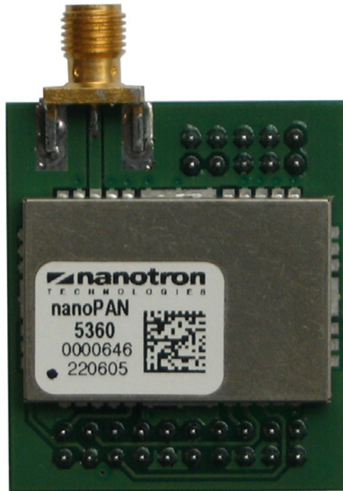
Figure 11: nanoPAN 5360 RF Module Adapter Board
