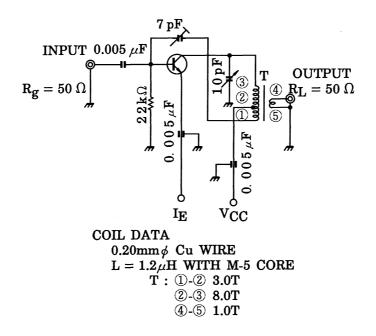
Figure 1 45 MHz Gpe Test Circuit
