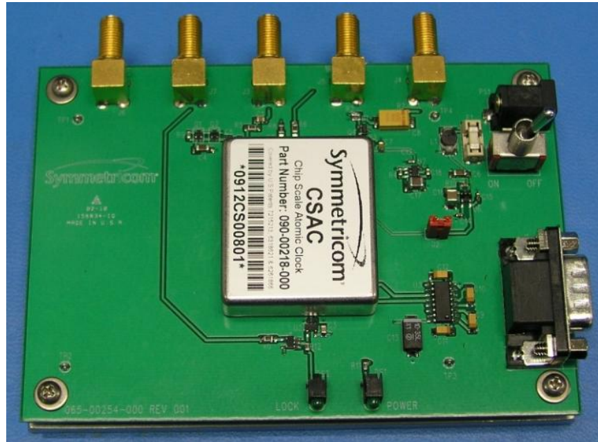
Figure 2: CSAC on evaluation board
