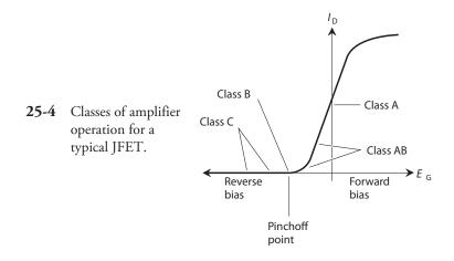
Engineers sometimes specify two distinct modes of class-AB amplification. If the bipolar transistor or FET never goes into cutoff or pinchoff during any part of the input signal cycle, the amplifier works in *class*  $AB_1$ . If the device goes into cutoff or pinchoff for any part of the cycle (up to almost half), the amplifier operates in *class*  $AB_2$ .
