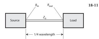
A quarter-wave matching section of transmission line. The input impedance equals  $R_{in}$ , the output impedance equals  $R_{out}$ , and the characteristic impedance equals  $Z_o$ .
