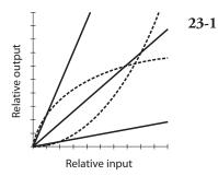
In a linear IC, the relative output is a linear (straightline) function of the relative input. The solid lines show examples of linear IC characteristics. The dashed curves show functions that aren't characteristic of properly operating linear ICs.
