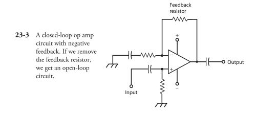
amplifier. Open-loop op amps sometimes exhibit instability, especially at low frequencies, breaking unexpectedly into oscillation. Open-loop op-amp circuits also generate significant internal noise, which can cause trouble in some applications.
