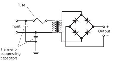
**24-13** A full-wave bridge rectifier with transient-suppression capacitors and a fuse in the transformer primary circuit.
