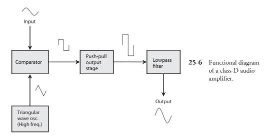
in Chap. 27 (Wireless Transmitters and Receivers) and Chap. 29 (Microcontrollers). Figure 25-6 shows the principle of class-D operation.
