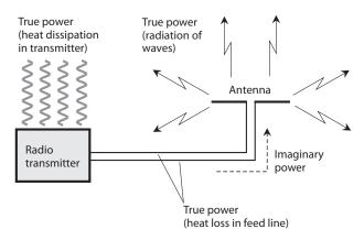
17-3 True power and imaginary power in a radio transmitter and antenna system.
