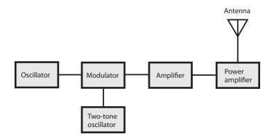
**27-1** Simplified block diagram of a transmitter that uses audio-frequency-shift keying (AFSK).
