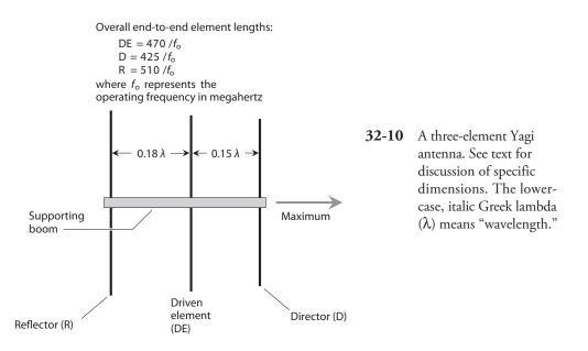
represent electrical dimensions (taking the velocity factor of wire or tubing into account), and not free-space dimensions.
