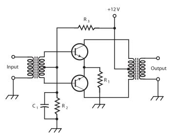
25-5 A class-B push-pull amplifier using NPN bipolar transistors.
