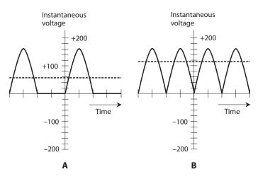
**2-10** At A, half-wave rectification of common utility AC. At B, full-wave rectification of common utility AC. Effective voltages are shown by the dashed lines.
