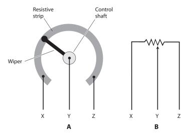
**6-8** Simplified functional drawing of a rotary potentiometer (A), and the schematic symbol (B).
