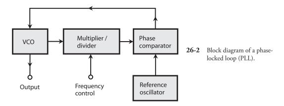
As you might expect, dedicated ICs are also available that can control the output frequency of an oscillator using a control voltage.
