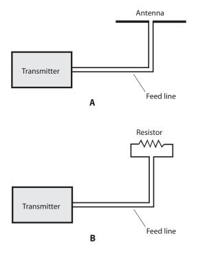
**6-3** At A, a radio transmitter connected to a real antenna. At B, the same transmitter connected to a resistive "dummy" antenna.
