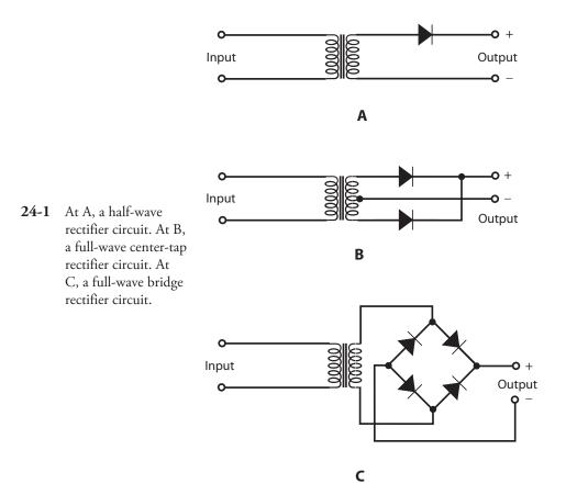
the equipment connected to it. The main advantage of a half-wave circuit is the fact that it costs less than more sophisticated circuits because it contains fewer parts.
