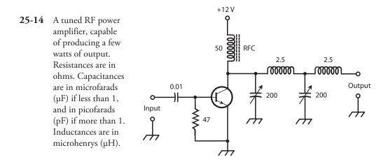
Tuned PAs can work into a wide range of load impedances. In addition to a *tuning control*, or resonant circuit that adjusts the output of the amplifier to the operating frequency, the tuned amplifier incorporates a *loading control* that optimizes the signal transfer between the amplifier and the load (usually an antenna).
