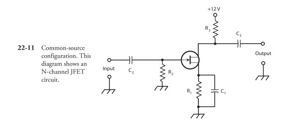
positive power supply terminal. For P-channel devices, the schematics would be the same except that the supply would provide a negative, rather than a positive, voltage.
