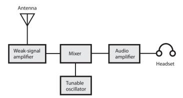
**27-10** Block diagram of a direct-conversion receiver.
