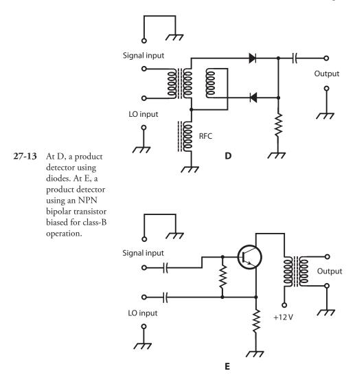
lies in the nonlinearity of the semiconductor devices. This nonlinearity facilitates the heterodyning necessary to obtain sum and difference frequency signals that result in data output.
