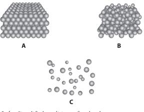
**1-4** Simplified renditions of molecular arrangements in a solid (A), a liquid (B), and a gas (C).
