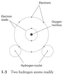
1-3 I wo hydrogen atoms readily share electrons with a single atom of oxygen.
