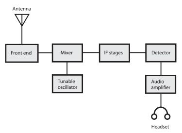
27-11 Block diagram of a single-conversion superheterodyne receiver.
