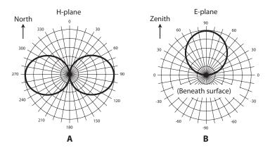
**32-6** Directivity plots for a dipole. At A, the H-plane (horizontal plane) plot as viewed from high above the antenna. Coordinate numbers indicate compass-bearing (azimuth) angles in degrees. At B, the E-plane (elevation plane) plot as viewed from a point on the earth's surface far from the antenna. Coordinate numbers indicate elevation angles in degrees above or below the plane of the earth's surface.
