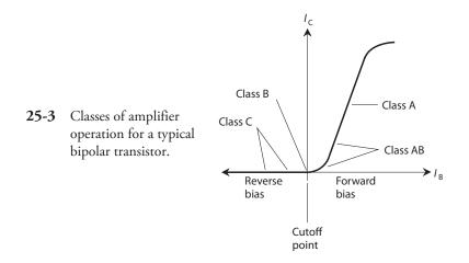
the characteristic curve during part of the cycle. When this phenomenon occurs, the output waveform will no longer represent a faithful reproduction of the input waveform, and the amplifier will become *nonlinear*. In some types of amplifiers, we can tolerate (or even encourage) nonlinearity, but we'll want a class-A amplifier to operate in a linear fashion at all times.
