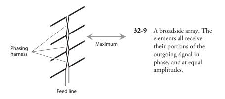
design the *phasing system* (also called the *phasing harness*), we must cut the branches of the transmission line to precisely the correct lengths, taking the velocity factor of the line into account.
