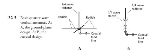
You've seen ground-plane antennas if you've spent much time around *Citizens Band* (CB) fixed radio installations that operate near 27 MHz, or if you've done much amateur-radio activity in the very-high-frequency (VHF) bands at 50 or 144 MHz.
