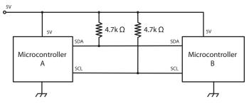
**29-9** Microcontroller-to-microcontroller communication using I<sup>2</sup>C.
