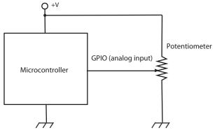
**29-7** Attaching a potentiometer to the analog input of a microcontroller.
