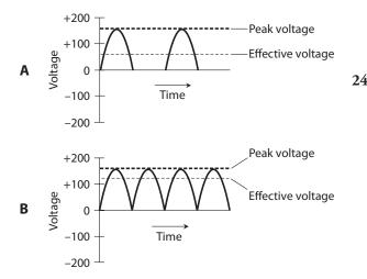
24-2 At A, the output of a half-wave rectifier. At B, the output of a full-wave rectifier. Note the difference in how the effective voltages compare with the peak voltages.
