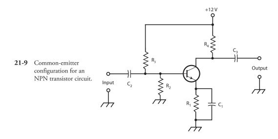
variations in  $I_{\rm B}$ . These small current fluctuations produce large variations in the current through R<sub>4</sub>. Therefore, amplification occurs. The output wave follows along in phase with the input wave.
