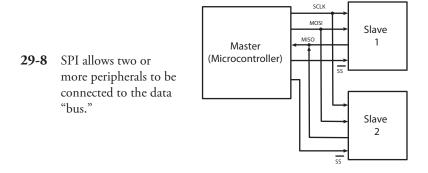
the slave device, and *Master In Slave Out* (MISO) the reverse. A separate clock signal synchronizes the data transmission.
