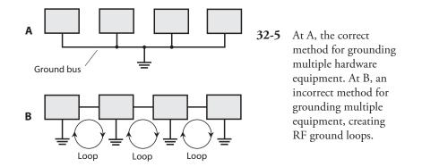
lightning strikes in the vicinity. A good electrical ground also minimizes the risk of *electromagnetic interference* (EMI) to and from radio equipment. In a three-wire electrical utility system, the ground prong on the plug should never be defeated because such modification can result in dangerous voltages appearing on exposed metal surfaces.
