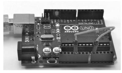
**30-7** An Arduino measuring its own voltages.
