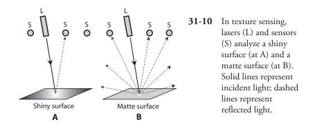
surface as either shiny or matte. The determination can also be affected by the motion of the sensor relative to the surface. A surface interpreted as shiny when standing still relative to the sensor might be interpreted as matte when moving relative to the sensor.
