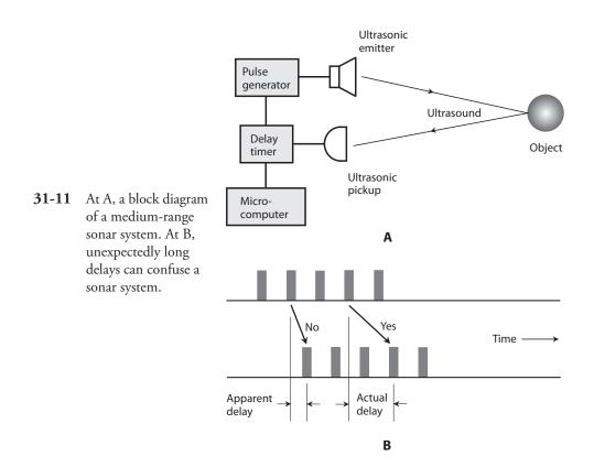
1400 meters per second (m/s), or 4600 feet per second (ft/s). In salt water, acoustic waves travel at about 1500 m/s (4900 ft/s). In air, acoustic waves travel at approximately 335 m/s (1100 ft/s).
