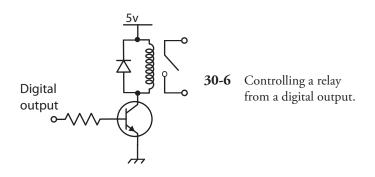
Figure 30-6 shows the use of an NPN bipolar transistor to provide the 50 to 100mA (or so) needed to drive the coil of a typical relay. The resistor should limit the current to less than 40mA, so 150  $\Omega$  would be ideal. A simple low-cost transistor, like the 2N3904, is suitable. The diode across the relay coil is necessary to snub (that is, suppress) any pulses of voltage resulting from driving the inductive load of the relay coil.
