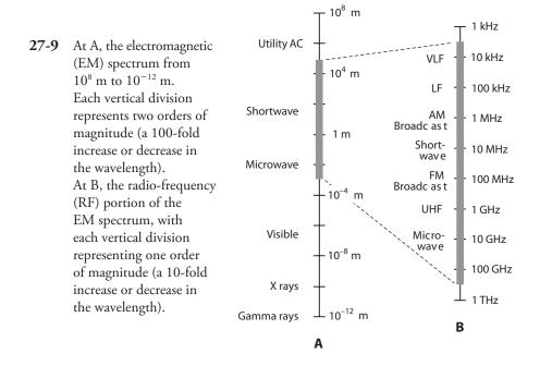
according to frequency. The RF spectrum is categorized in *bands* from *very low frequency* (VLF) through *extremely high frequency* (EHF), according to the breakdown in Table 27-1. The exact lower limit of the VLF range is a matter of disagreement in the literature. Here, we define it as 3 kHz.
