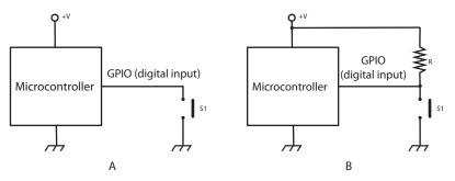
**29-4** Connecting a switch to a digital input.
