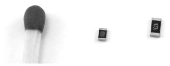
**6-10** SMD resistors with match for scale.
