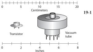
A power-amplifier transistor (at left) has much smaller volume and mass than a vacuum tube of comparable signaloutput capacity (right).
