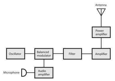
27-6 Block diagram of a basic SSB transmitter.
