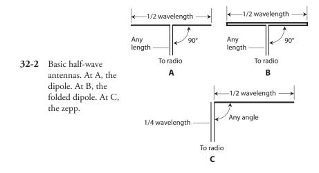
half-wave open dipole made from a single wire. This "resistance-multiplication" property makes the folded dipole ideal for use in parallel-wire transmission lines, which usually have high characteristic impedance ( $Z_o$ ) values.
