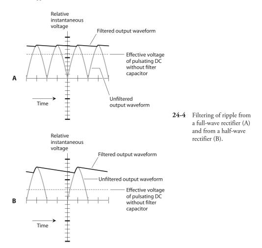
output gives the capacitor a "less bumpy ride," while the half-wave output lets the capacitor discharge more between each "refresh pulse."
