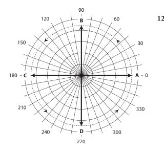
12-5 Rotating-vector representation of a sine wave. Vector A portrays the start of the cycle  $(0^\circ)$ ; vector **B** portrays the wave <sup>1</sup>/<sub>4</sub> of the way through the cycle (90°); vector **C** portrays the wave halfway through the cycle (180°); vector **D** portrays the wave <sup>3</sup>/<sub>4</sub> of the way through the cycle (270°). The vector length never changes.
