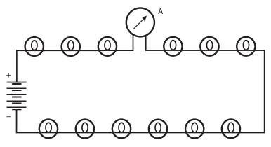
5-1 Light bulbs in series, with an ammeter (A) in the circuit.
