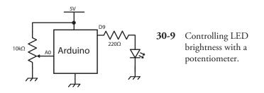
The sketch for this project simply takes the analog reading from the potentiometer (0 to 1023) and divides it by 4 to put it in the range 0 to 255 needed by analogWrite.
