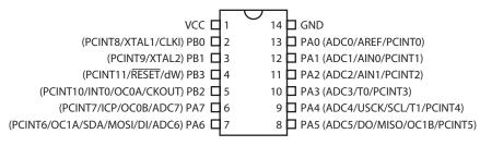
**29-12** The pinout of an ATtiny44.
