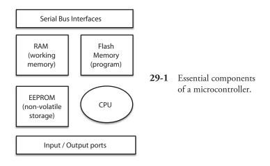
"Digital Basics." However, because what links the pins is software rather than, say, a hardware AND gate, the microcontroller is almost infinitely flexible, limited only by its speed, memory, and the ability of you, the programmer, to write the program that controls it.
