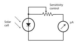
**3-11** A simple light meter with a potentiometer to adjust the sensitivity.
