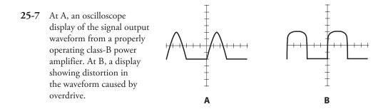
taking place in a particular situation. The scope gives us an instant-to-instant graphical display of signal amplitude as a function of time. We connect the scope to the amplifier output terminals to scrutinize the signal waveform. The output waveform for a particular class of amplifier always has a characteristic shape; overdrive causes a form of distortion known as *flat topping*.
