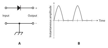
**20-1** At A, a half-wave rectifier circuit. At B, the output of the circuit shown at A when we apply an AC sine wave to the input.
