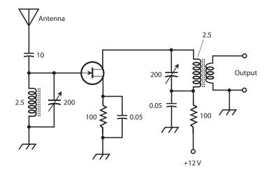
**25-12** A tuned RF amplifier for use at approximately 10 MHz. Resistances are in ohms. Capacitances are in microfarads  $(\mu F)$  if less than 1, and in picofarads (pF) if more than 1. Inductances are in microhenrys  $(\mu H)$ .
