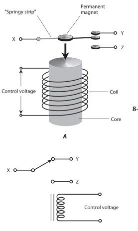
**8-6** Simplified drawing of a relay (at A) and the schematic symbol for the same relay (at B).
