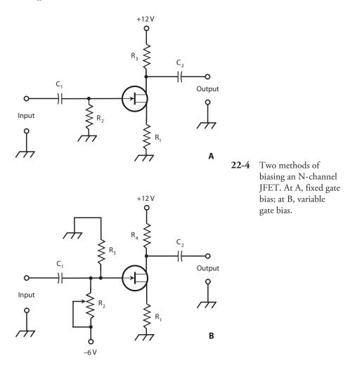
weak-signal amplifiers, low-level amplifiers, and oscillators. The scheme at B works well in power amplifiers having substantial input signal amplitudes.
