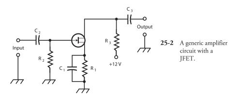
The optimum resistor values also depend on the application. In the case of a weak-signal amplifier, typical values are 470  $\Omega$  for R<sub>1</sub>, 4.7 k for R<sub>2</sub>,10 k for R<sub>3</sub>, and 4.7 k for R<sub>4</sub>.
