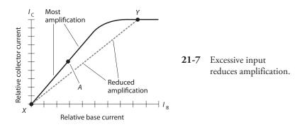
output wave does not have the same shape as the input wave. We call this phenomenon *nonlinearity*. We can sometimes tolerate this condition, but often it's undesirable. Under most circumstances, we'll want our amplifier to remain *linear* (or to exhibit excellent *linearity*), meaning that the output wave has the same shape as (although probably stronger than) the input wave.
