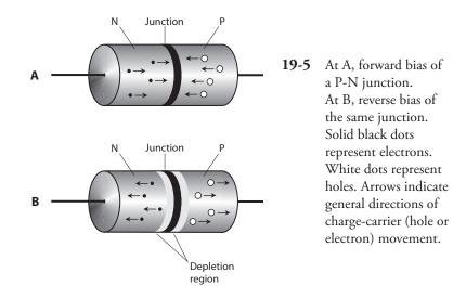
A reverse-biased P-N junction forms a capacitor. Some semiconductor components, called *varactor diodes*, are manufactured with this property in mind.
