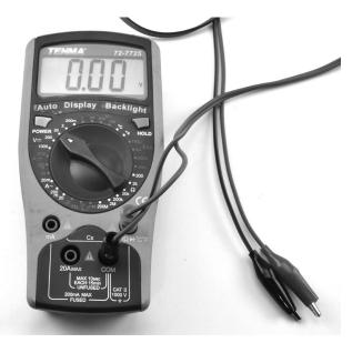
**3-10** A low-cost digital multimeter.
