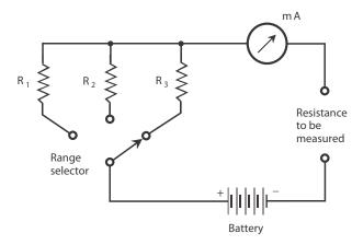
**3-8** A circuit using a milliammeter (mA) to measure DC resistance.
