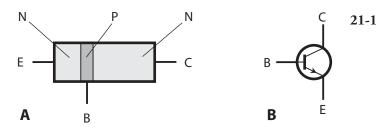
At A, a simplified structural drawing of an NPN transistor. At B, the schematic symbol.
