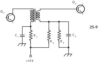
5-9 An example of transformer coupling between amplifier stages. signal ground. Resistor  $R_1$  limits the current through the first transistor  $Q_1$ . Resistors  $R_2$  and  $R_3$  provide the base bias for transistor  $Q_2$ .
