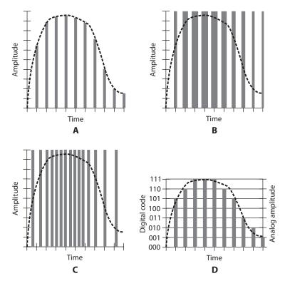
**27-8** Time-domain graphs of various modes of pulse modulation. At A, pulse-amplitude modulation (PAM); at B, pulse-width modulation (PWM), also called pulse-duration modulation (PDM); at C, pulse-interval modulation (PIM); at D, pulse-code modulation (PCM).
