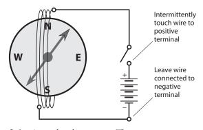
**3-1** A simple galvanometer. The magnetic compass must lie flat.
