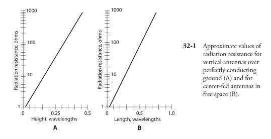
always appears in series with a certain *loss resistance* ( $R_L$ ). We can calculate the antenna efficiency, *Eff*, as a ratio with the formula  $Eff = R_R / (R_R + R_I)$
