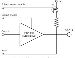
**29-2** Simplified schematic of a GPIO pin.
