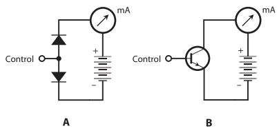
**21-3** At A, the dual-diode model of a simple NPN circuit. At B, the actual transistor circuit.
