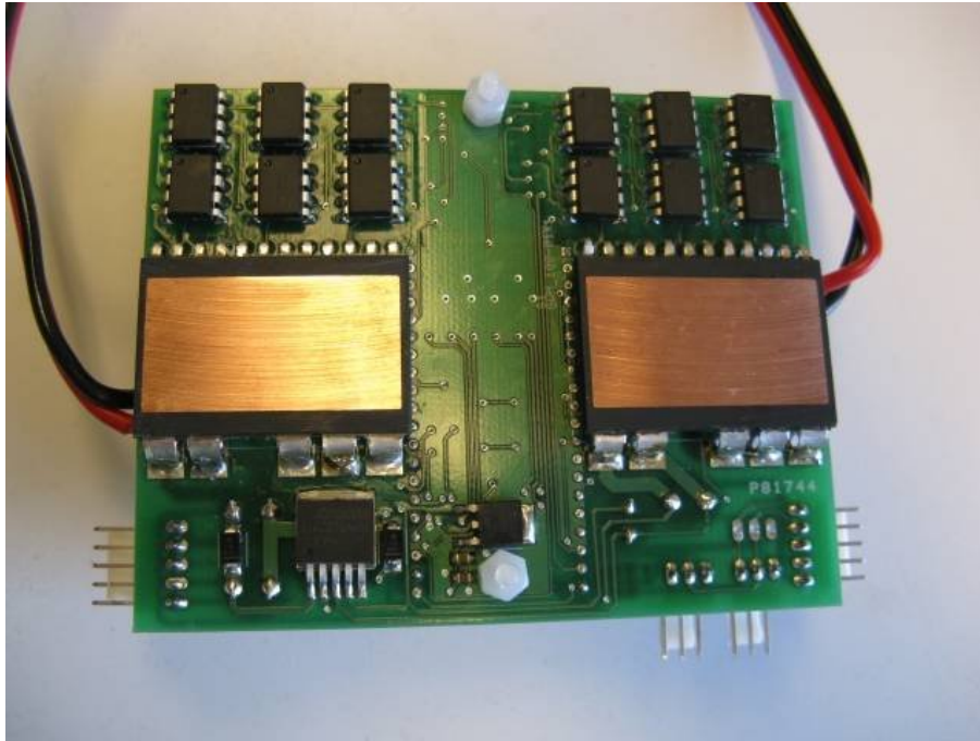
Figure 54: Two IXYS GWM 100-01X1 modules installed on the bottom side of the scooter controller.
