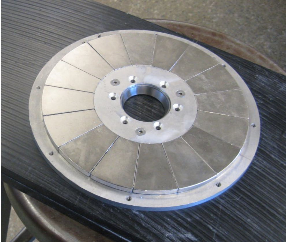
Figure 23: Each magnet disk has 16 NdFeB magnets that form an 8" OD and 4" ID region of magnetization. The magnets are 0.25" in thickness and backed by 0.25" steel.
