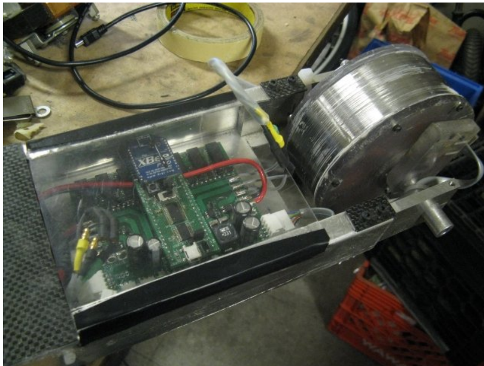
Figure 48: The latest version of the case study controller, which fits entirely within the scooter deck. It is capable of full sinusoidal field-oriented control of both scooter motors simultaneously.
