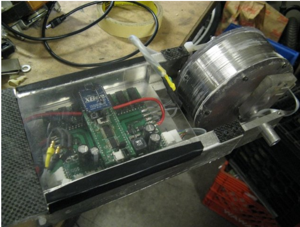
Figure 63: The v2.1 controller fits under a transparent cover flush with the scooter deck, so it does not occupy foot space. It is heat sinked directly to the aluminum chassis.
