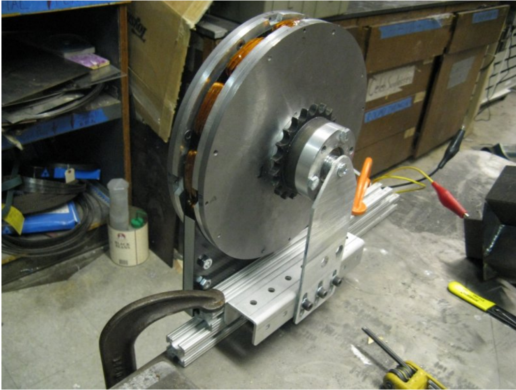
Figure 26: The coreless axial flux motor prototype build for this case study.
