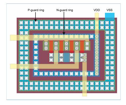
It is generally believed that N-well guard ring in P-substrate and Pdiffusion guard ring in N-well are not of much use. The stray electrons and holes travel deep into the substrate and are not collected by the guard rings. However, putting a guard ring is better than leaving the space empty since we still have to keep the noisy transistors at a distance away from the other transistors.
