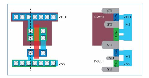
Two alternative layouts are shown below. The p-tap is butted with the ndiffusion, and the n-tap is butted with the p-diffusion. The trade-off in the new layouts is a larger area.
