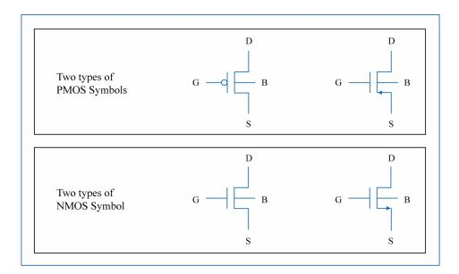
The bulks of the PMOS and the NMOS are usually connected to power and ground respectively. If the bulk terminal is omitted from the schematic symbol, the connections can be assumed to be what is shown in the following diagram.
