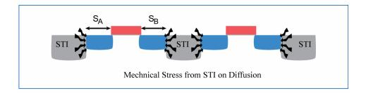
To reduce the effect of STI stress, the source and drain diffusions require to be extended when they are next to the STI. However, a large diffusion also increases parasitic capacitance and layout area. A better approach is to insert one or more dummy transistors at each end of the transistor as illustrated in the diagram below. Note that the dummy transistor must share the diffusion with the non-dummy transistor.
