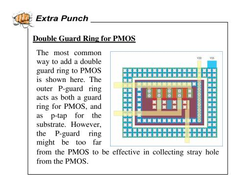
An important layout practice is to ensure that there is no (or very little) current flowing through any part of the guard ring. Consider the layout in the diagram below. A current flowing in the p-type guard ring raises its potential above VSS. If the potential of the n-diffusion next to the p-type guard ring (shaded in the diagram) is at VSS, the PN junction potentially becomes forward biased, and results in holes injected from the guard ring into the substrate!
