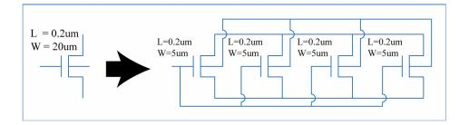
The next layout shows the transistor with four fingers. The layout has a better aspect ratio than the one in the first stroke. Note that the connection to the bulk is omitted in the layout so as to simplify the drawing. Bulk connection will be discussed later.
