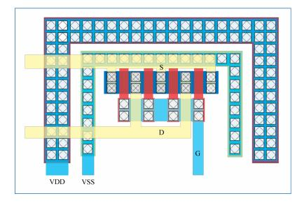
If reducing the area of the layout is of utmost priority and you do not expect much minority carrier noise in the silicon, then you may consider reducing the numbers of local N-well guard rings and P-diffusion guard rings.
