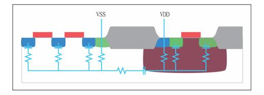
To reduce disturbances from minority carrier, you may use guard ring in the following configuration around noisy transistors.
