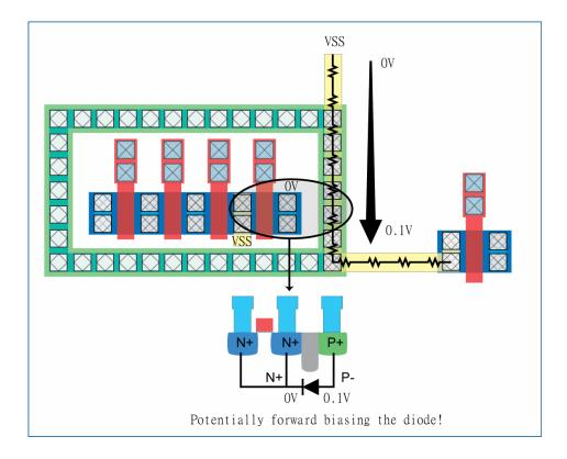
A more subtle case is shown below. In the circuit design, the source of the transistor is connected to VSS. It is very convenient to tap the VSS from the guard ring as shown in the layout below. If the peak current going through the transistor is very small, the layout may be acceptable. Otherwise, tapping power from the guard ring is not allowed.
