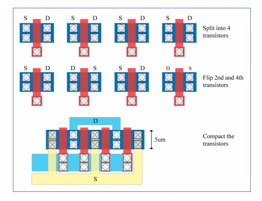
So far everything looks fine. **But it is not**. The transistor with a width of 20um and a length of 0.2um is not exactly the same as having four transistors that are connected in parallel, each with a width of 5um and a length of 0.2um.
