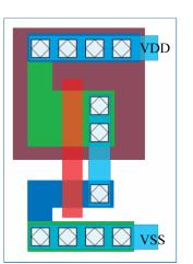
a deposited metal is reacted thermally with the poly and the diffusion to form silicide. When the p-diffusion and the n-diffusion are butted, they are connected by the layout of silicide above them!
