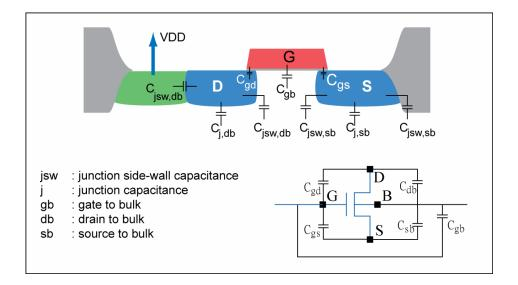
Overall  $C_{sb}$  is dependent on the area of source (AS) and perimeter of source (PS). Similarly, overall  $C_{db}$  is dependent on the area of drain (AD) and perimeter of drain (PD). Both  $C_{sb}$  and  $C_{db}$  have components that are dependent on the diffusions in the proximity. The values of AS, AD, PS and PD of a transistor can be extracted from the layout. Post-layout spice netlist should include these parameters.
