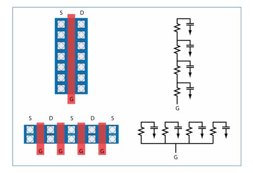
In general, try to fold a transistor to an even number of fingers. For example, the transistor from the second stroke is folded to four transistors, and is drawn to optimize the frequency response of the drain.<sup>1</sup>
