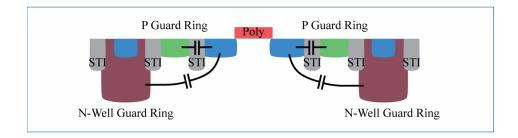
Instead of using a full guard ring, you may consider using a U-shape guard ring. Some circuit designers do not favor the use of U-shape guard ring while some circuit designers use U-shape guard ring only for the p-tap and the n-tap. The following layout shows a NMOS with U-shape guard rings.
