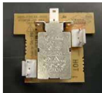
MAIN POWER SWITCH CONTROL
