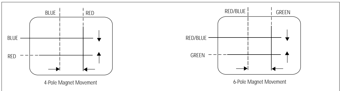
Fig. 4-5 Center Convergence Adjustment
