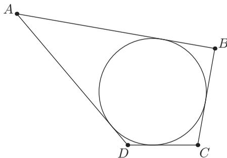
**Figure 2.8A.** The Pitot theorem:  $AB + CD = BC + DA$ .
