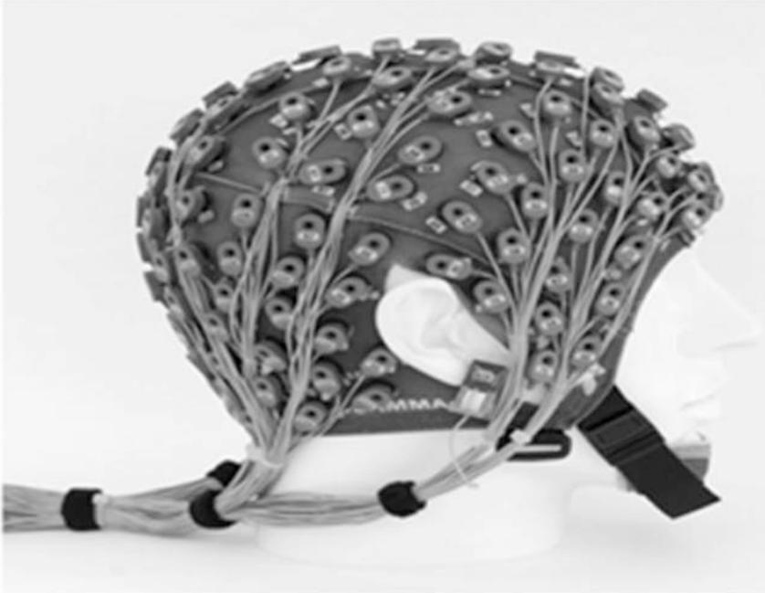
**FIGURE 5.6** A 256-channel EEG cap.
