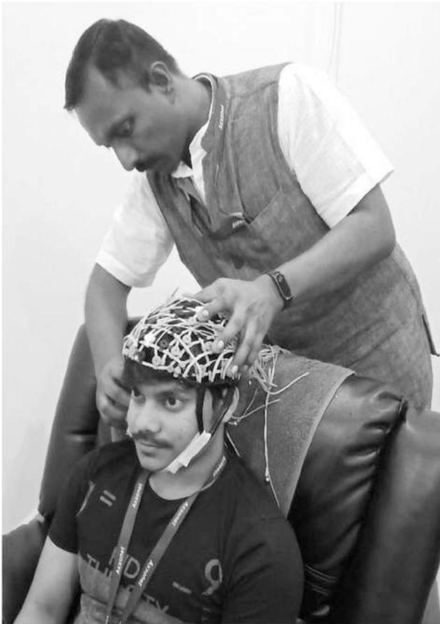
**FIGURE 6.3** Subject wearing EEG cap while recording of EEG and EOG signal. (Courtesy Axxonet Pvt. Ltd., Bangalore, India.)
