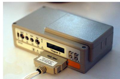
Portable recording device for EEG
