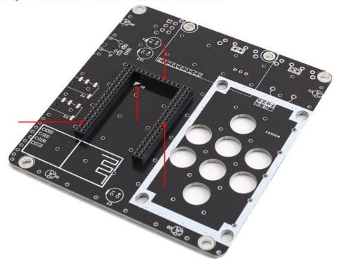
Step 3: Install 1pcs Green Main IC Controller Module on Female Pin which has been install on step 2.
