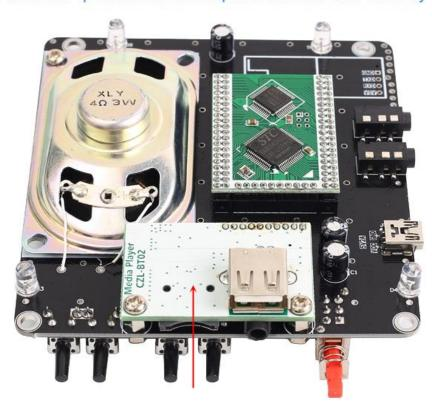
Step 14: Install 1pcs Bluetooth Amplifier Module and fixed by screw.
