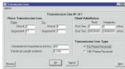
Figure 6—The NEC-Win Plus screen for introducing a mathematical transmission line into a model.
