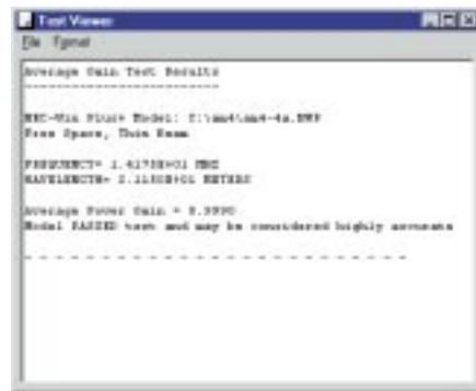
Figure 10—The NEC-Win Plus report on the results of the average gain test for the 3-element Yagi used for the beta-match illustration.
