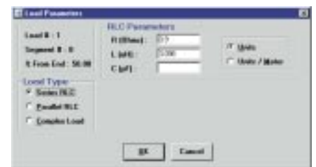
Figure 4—The NEC-Win Plus basic entry screen for loads consisting of a resistance and an inductance in series. A series capacitor, not used in this example, could be added to the mixed load. Note that parallel combinations of resistance, inductance and capacitance are also possible.
