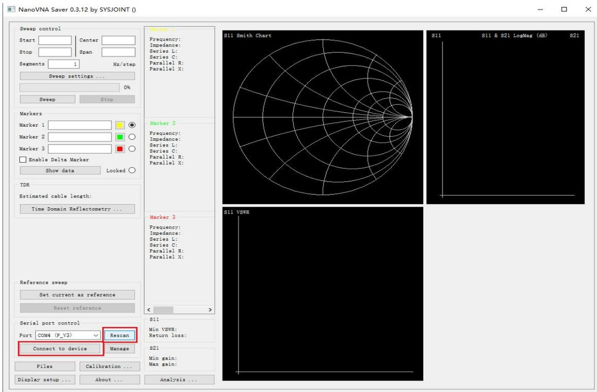
Through the PC software, you can set the start and stop frequency, get the measurement results, set the marker, take a screenshot, etc.
