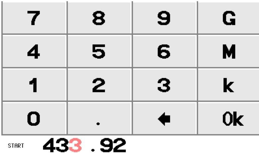
The virtual keyboard includes numeric keys, backspace key, unit key, ok key.
