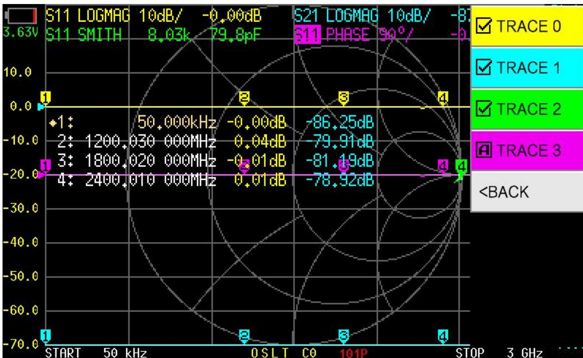
Tap on [TRACE n] (e.g., [TRACE 2] ) will open and activate TRACE 2, and an  marker will appear ahead of "TRACE 2". Tap on another menu item (e.g., [TRACE 3]) will open and activate TRACE 3, at this time, an  marker will appear ahead of "TRACE 3", and the  marker ahead of "TRACE 2" becomes , which means TRACE 2 and TRACE 3 are both opened and TRACE 3 is current active.
