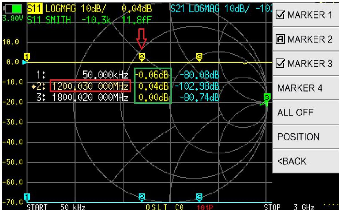
Tap on [MARKER n] (e.g., [MARKER 2]) will open and activate MARKER 2, and an  marker will appear ahead of "MARKER 2". Tap on another menu item (e.g., [MARKER 3]) will open and activate MARKER 3, at this time, an  marker will appear ahead of "MARKER 3", and the  marker ahead of "MARKER 2" becomes , which means MARKER 2 and MARKER 3 are both
