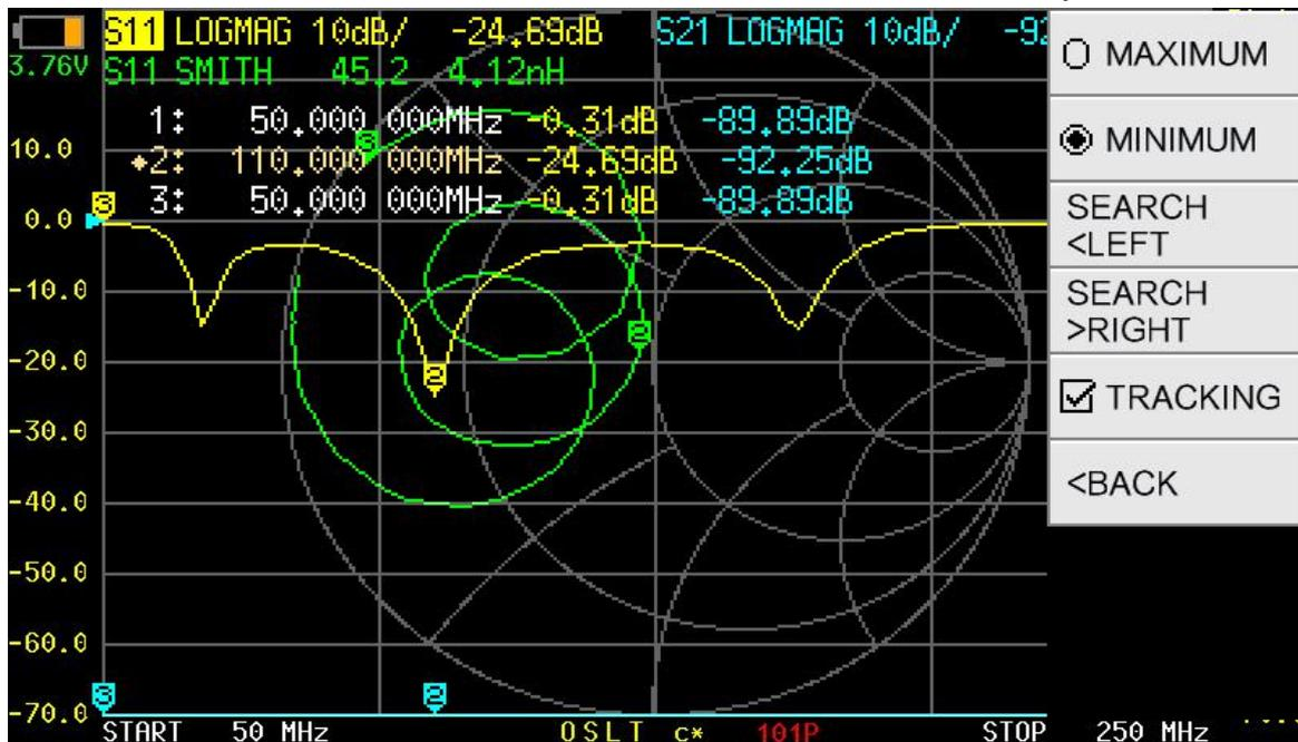
**[TRACKING]** is used to automatically track the maximum or minimum value of the trace. As shown in the figure above, if you want MARKER 2 to automatically track the minimum value of the S11 LOGMAG trace, firstly you should activate MARKER 2, and then tap on **[MINIMUM]** , and finally turn on **[TRACKING]** . After doing that, MARKER 2 will automatically move to the
