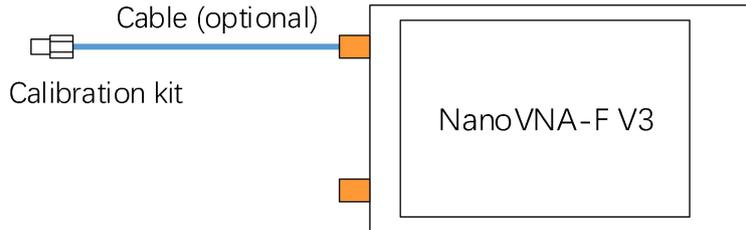
Tap on **[OPEN]**, the device emits a beep, and the menu turns gray and is inoperable. Wait for 2-3 seconds, the device emits a beep again, an
