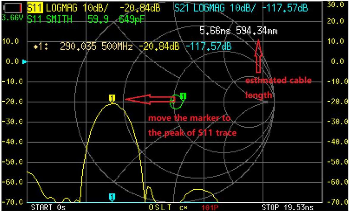
There are 3 kinds of digital processing mode available: **[LOW PASS IMPULSE]** , **[LOW PASS STEP]** , **[BANDPASS]** , and default setting is **[BANDPASS]** .
