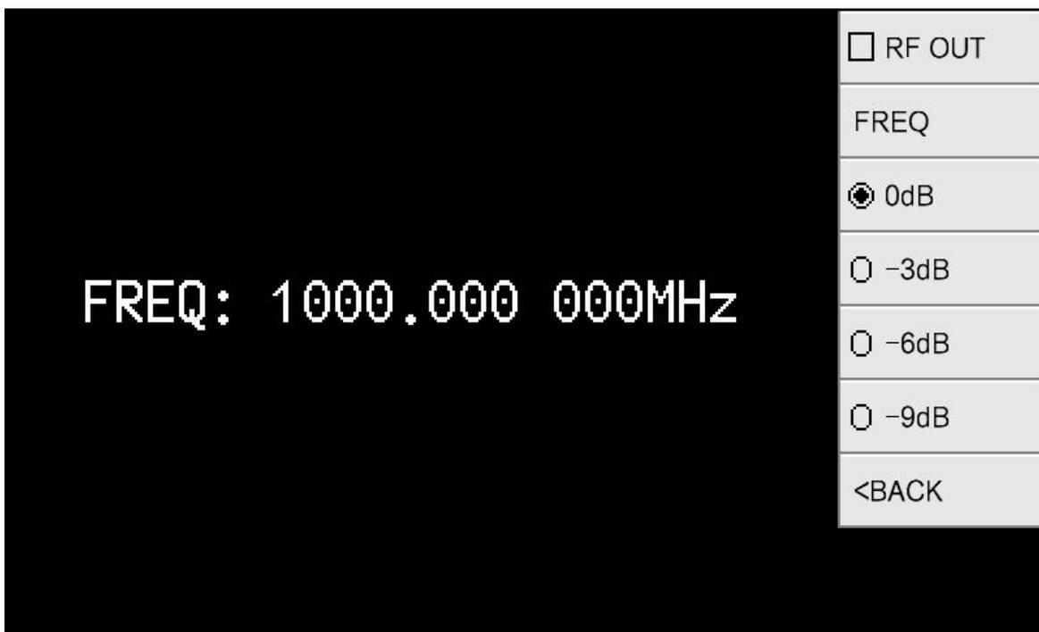
**[SIGNAL GENERATOR]** NanoVNA-F V3 supports simple signal generator function, which can be set as a single-frequency continuous wave generator with a frequency range from **1MHz** to **6000MHz**. RF power is adjustable above **23.5MHz**.
