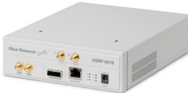
The following two block diagrams apply to the N210 and RFX2400 respectively. RF signals apparent at the antenna are down-converted in quadrature with dedicated hardware on the RFX2400 and presented to the N210 at baseband (zero-IF). The quadrature ADC on the N210 samples at 100 Msps which is fed into the FPGA. The main signal processing blocks of the N210 FPGA are described in Appendix C. The FPGA provides the resulting samples as an ethernet stream on the N210 gigabit ethernet port.
