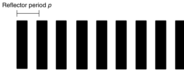
Figure 4.94 Geometry of a simple reflector for surface waves (reproduced by permission of Siemens AG, ZT KM, Munich)
