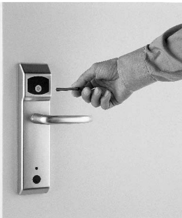
Figure 13.17 Offline terminal integrated into a doorplate. The lock is released by holding the authorized transponder in front of it. The door can then be opened by operating the handle. The door terminal can be operated for a year with four 1.5 V Mignon batteries and even has a real time clock that allows it to check the period of validity of the programmed data carrier. The terminals themselves are programmed by an infrared data transmission using a portable infrared reader (reproduced by permission of Häfele GmbH, D-Nagold)
