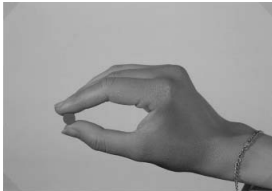
Figure 2.7 Transponder in a standardised construction format in accordance with ISO 69873, for fitting into one of the retention knobs of a CNC tool (reproduced by permission of Leitz GmbH & Co., Oberkochen)
