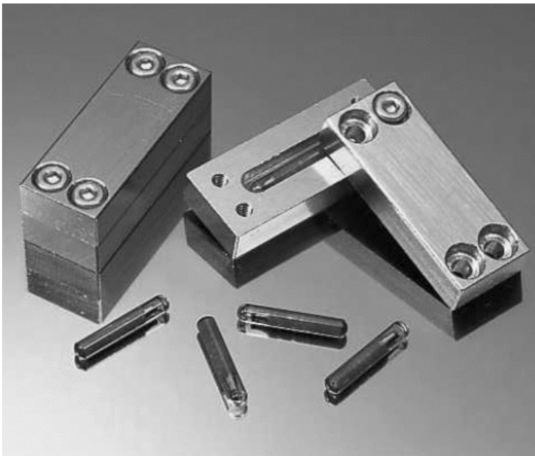
Figure 4.53 Right, fitting a glass transponder into a metal surface; left, the use of a thin dielectric gap allows the transponders to be read even through a metal casing (Photo: HANEX HXID system with Sokymat glass transponder in metal, reproduced by permission of HANEX Co. Ltd, Japan)
