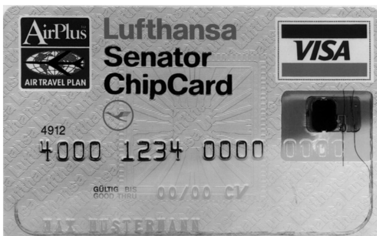
Figure 13.12 Miles & More — Senator ChipCard, partially cut away. The transponder module and antenna are clearly visible at the right-hand edge of the picture underneath the hologram (reproduced by permission of Giesecke & Devrient, Munich)
