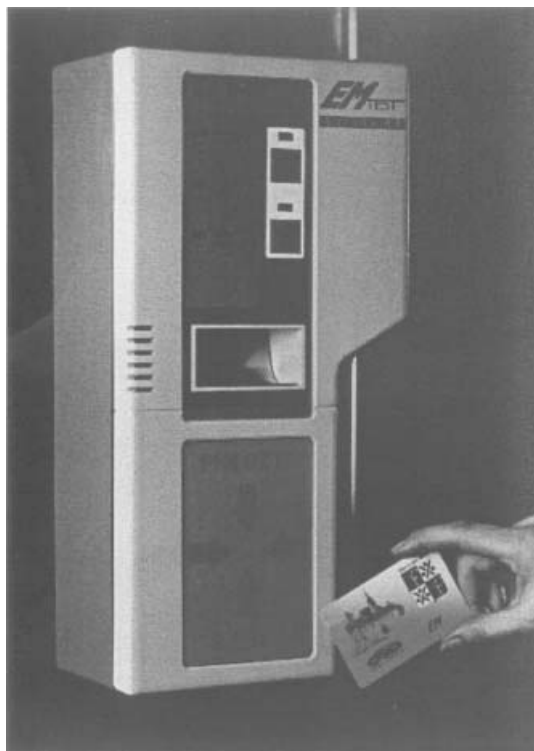
Figure 13.3 Contactless reader in a public transport system (photo: Frydek-Mistek project, Czechoslovakia, source: reproduced by permission of EM Test)
