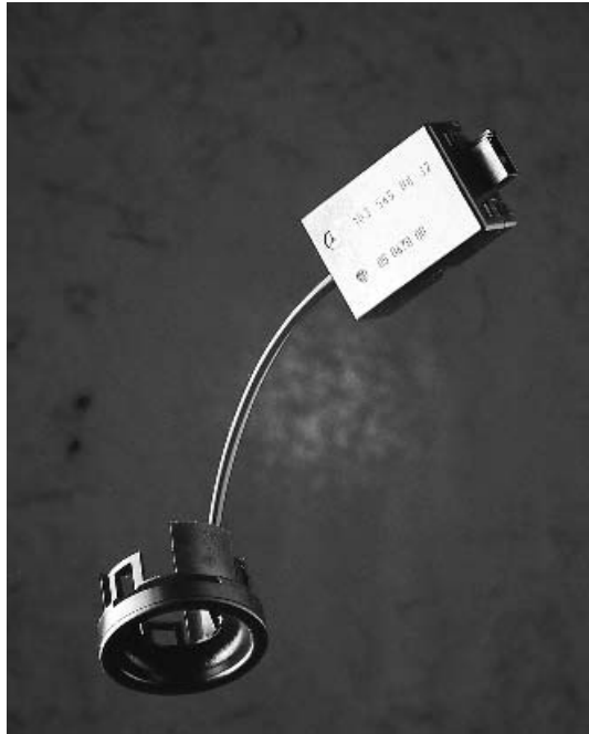
Figure 13.35 The antenna of the electronic immobilisation system is integrated directly into the ignition lock (reproduced by permission of Deister Elektronik, Barsinghausen)
