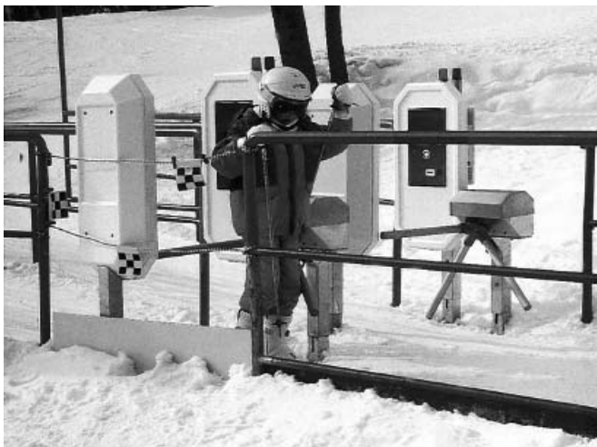
Figure 13.14 Contactless reader as access control and till device at a ski lift (reproduced by permission of Legic Identsystems, CH-Wetzikon)
