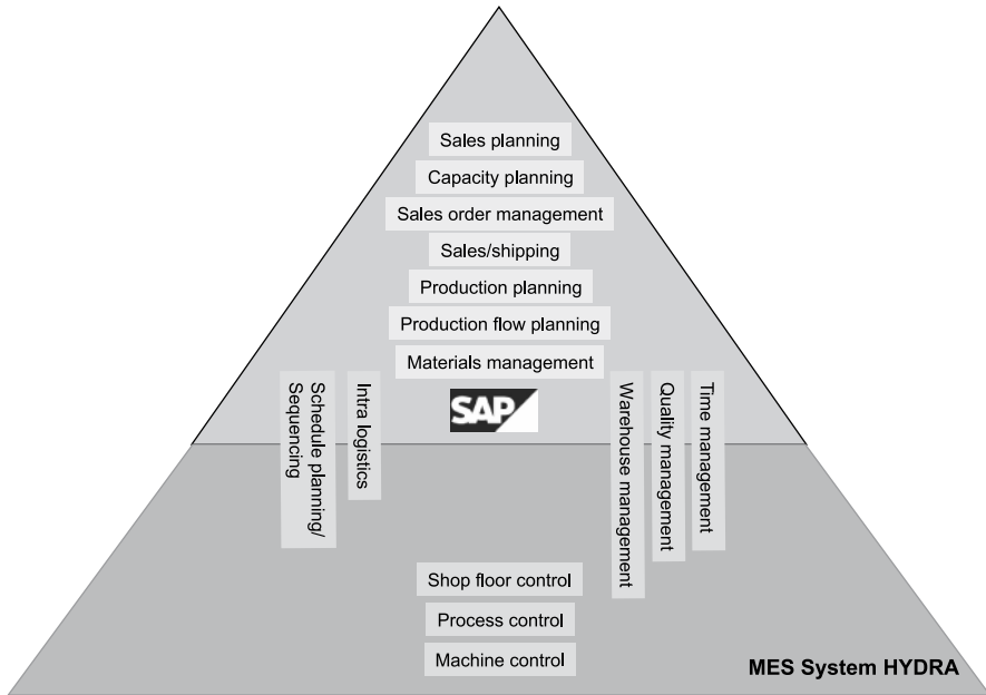
Fig. 3.3 Integration of a production company's processes into the IT environment
