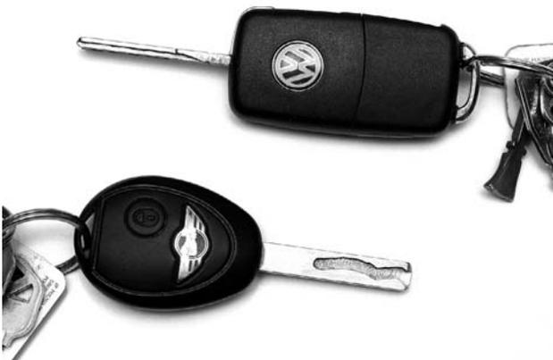
**FIGURE 3.9** LF tags are embedded in these keys
