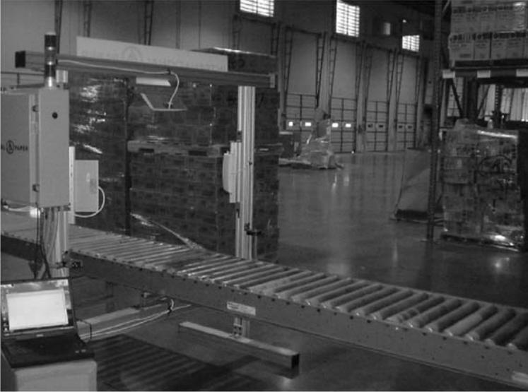
**FIGURE 7.4** Verification tunnel on a conveyor
