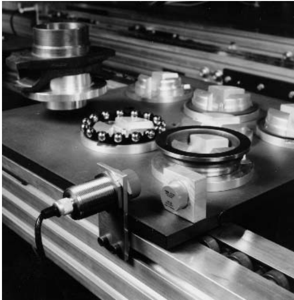
Figure 13.52 Individual components of a clutch release stop on a revolving pallet. Transponder and reader antenna are visible in the lower part of the photo (reproduced by permission of Pepperl & Fuchs, Mannheim)
