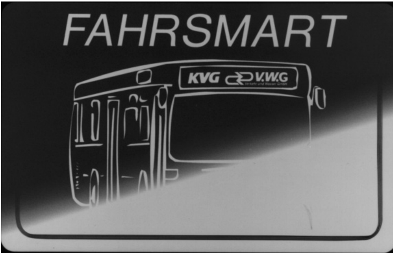
Figure 13.9 Fahrsmart II contactless smart card, partially cut away. The transponder coil is clearly visible at the lower right-hand edge of the picture (reproduced by permission of Giesecke & Devrient, Munich)
