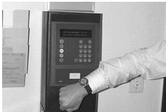
Figure 13.16 Access control and time keeping are combined in a single terminal. The watch with an integral transponder performs the function of a contactless data carrier (reproduced by permission of Legic® -Installation, Kaba Security Locking Systems AG, CH-Wetzikon)
