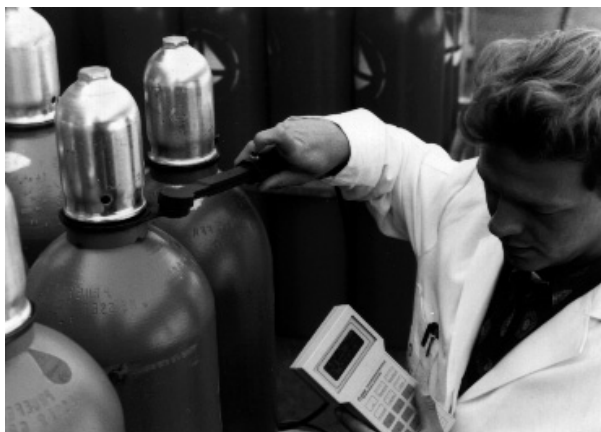
Figure 13.38 Identification of gas bottles using a portable reader. The reader (scemtec SIH3) is designed to function with transponders from different manufacturers (reproduced by permission of Messer Griesheim)
