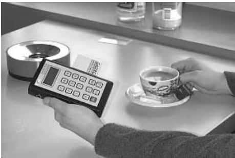
Figure 11.24 Reader for portable use in payment transactions or for service purposes. (Photo of LEGIC® reader reproduced by permission of Kaba Security Locking Systems AG, CH-Wetzikon)
